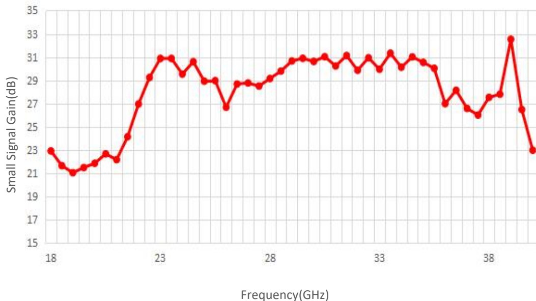
Small Signal Gain vs Frequency
